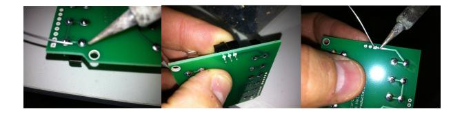
Now insert the Arduino style header connectors in the board one at a time. Again let the helping hand hold the solder while you use your two hands to solder the connector in place. Only solder one pin of the connector and then check it to make sure the connector is straight and perpendicular to the circuit board. Do this for each of the four connectors.
