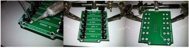
Solder both pads of each battery clamp on the bottom so all the battery clamps are solidly in place.
