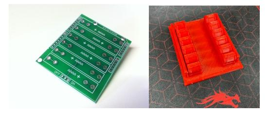
3D Print the base to hold the clips, install the board over the clips and solder the battery clips to the board.
