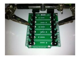
Solder each battery clip on the top side of the board with just enough to hold the clamp temporarily in place. Make sure the clamp is pushed as far to the outside of the board as possible while still keeping the tabs inside the holes.
